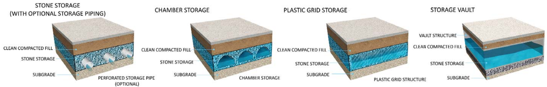
Figure 1-14. Infiltration/Storage Trench with Typical Features
