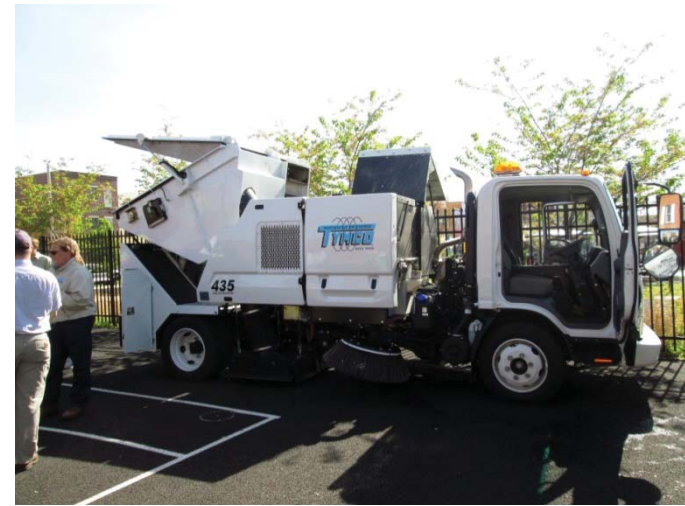
Figure 4-1. Regenerative Air Truck
