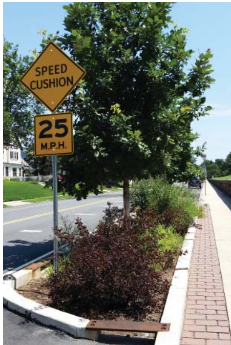
Figure 2-8. Tree with Elevated Lower Limbs to Preserve Sight Lines.
